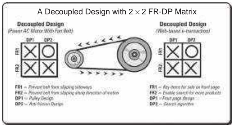
**EXHIBIT 31.3** A decoupled design is one in which all functional requirements can be achieved independently by adjusting design parameters. However, at least one design parameter affects two or more functional requirements.
