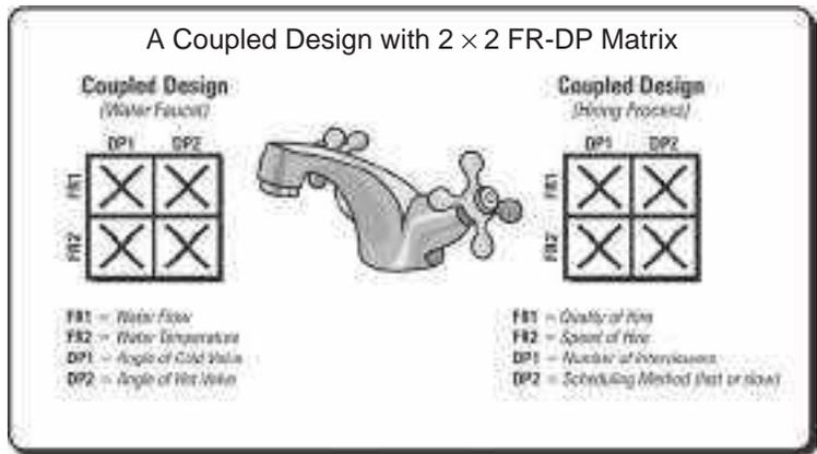
**EXHIBIT 31.2** A coupled design is one in which all functional requirements cannot be achieved independently by adjusting design parameters without affecting other functional requirements.
