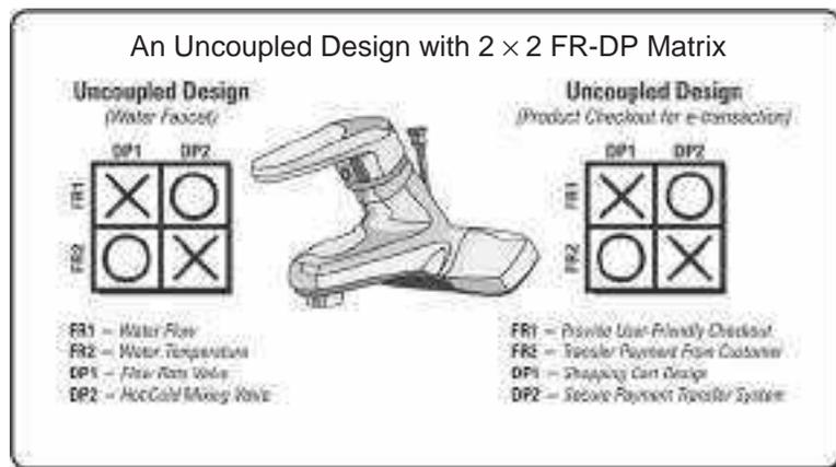
**EXHIBIT 31.4** An uncoupled design is one in which each functional requirement is independently achieved by a corresponding unique design parameter.
